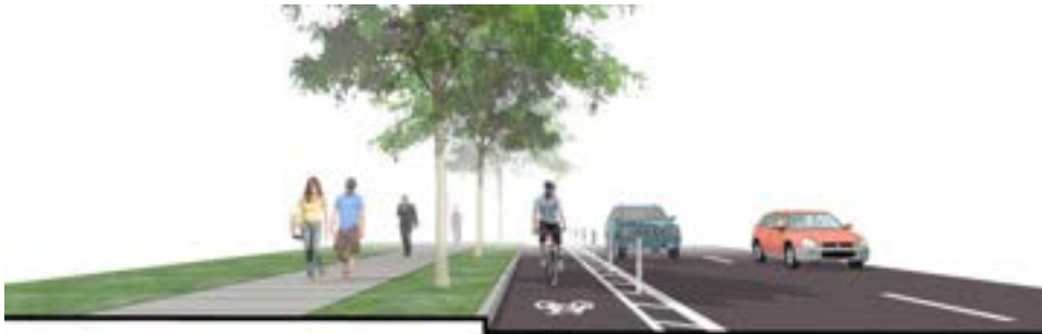
Figure 17: Buffered bike lane with vertical delineators
