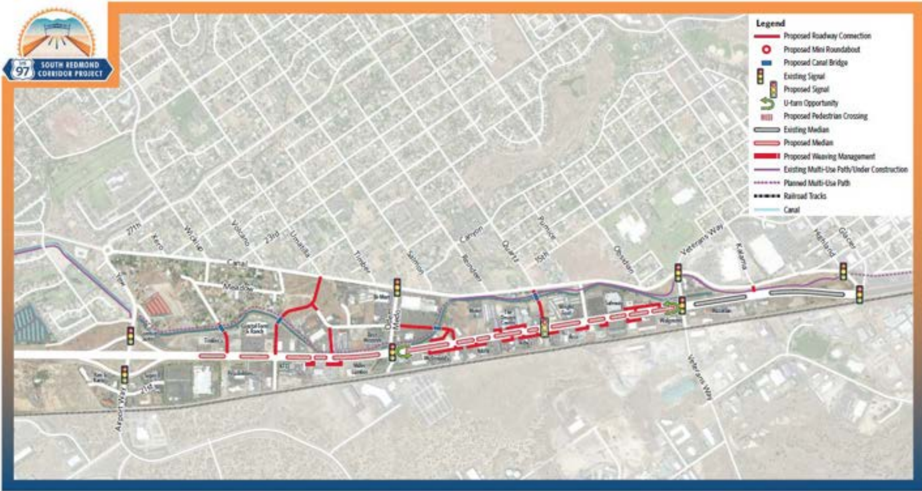
Figure 24. Concept B: Channelized Access and Circulation
