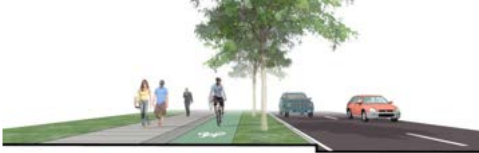
Figure 22: Sidewalk level cycle track
