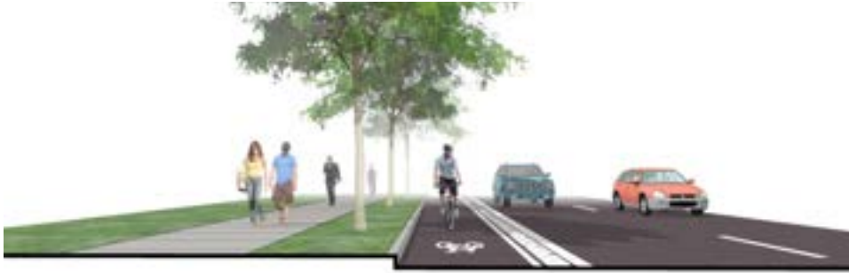
Figure 19: Protected bike lane with concrete curb
