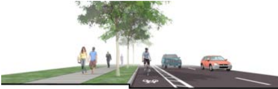
Figure 17: Buffered bike lane with vertical delineators
